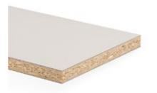
HPL bonded board consisting of a particleboard type P2 conforming to EN 312, surfaced on both sides with Duropal XTreme plus, an attractive supermatt surface material with an anti-fingerprint effect, which is ideal for horizontal, heavily used surfaces.
