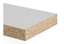
Worktop consisting of a particleboard type P2 conforming to EN 312, decor side surfaced with Duropal XTreme plus, underside with water-repellent backing. The longitudinal edges of the worktop are machined. It is also available as a variant with a protective edge on one longitudinal side. Duropal XTreme plus is an attractive supermatt surface material with an anti-fingerprint effect, which is ideal for horizontal, heavily-used surfaces.
