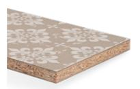
Flat bonded element with individually digitally printed motifs made from a particleboard core, Type P2 to EN 312, surfaced with Duropal HPL Individual Motiv, reverse side white. Our well-known Individual world from just 1 piece upwards, where your image files can be used as a motif.
