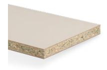
Flat bonded element of a moisture-resistant particleboard construction, Type P3 to EN 312, faced on both sides with Duropal HPL.
