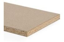
Chipboard bonded with 100 % biogenic, formaldehyde-free glue (OrganicGlue) with a recycled wood content of approx. 100 % type P2 according to EN 312, suitable for non-load-bearing purposes in dry areas.
