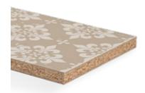
Urea resin bonded particleboard with individual digital print motifs in direct facing method, awarded with the Blue Angel. The front face is printed as required, the standard reverse is white.
