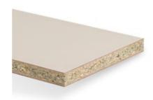
HPL bonded board consisting of a moisture-resistant particleboard type P3 to EN 312 for damp areas, surfaced on both sides with Duropal HPL.
