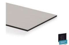
Compact high-pressure laminate for outdoor use in standard quality according to EN 438-6:EDS / intensive decors according to EN 438-6:EGS. With uniform black-coloured core and single-sided decorative acrylic lacquer on the top side and decorative melamine resin surface on the reverse or double-sided decorative acrylic lacquer.
