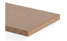
Urea resin-bonded particleboard, type P2 in accordance with EN 312, suitable for non load-bearing purposes in dry areas.
