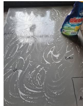
4. Apply the cleaning agent over the entire surface
